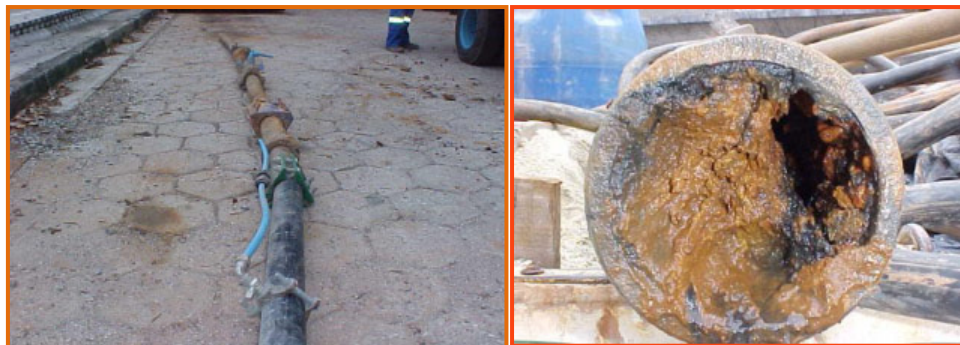
Figure 10 – Mains with high break frequency and crust.
