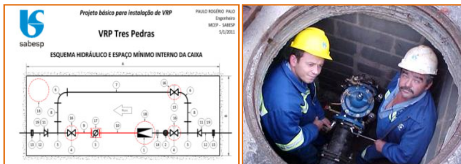
Figure 11- Tres Pedras PRV project and installation by Sabesp's team.
