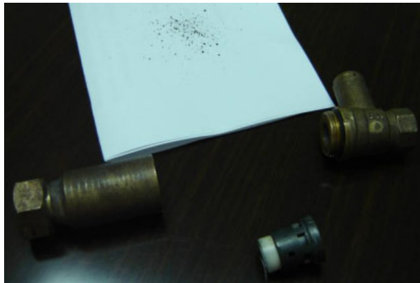
Figure 4 The rust and sand found in the drip-proof valve after used under the improved transformation
