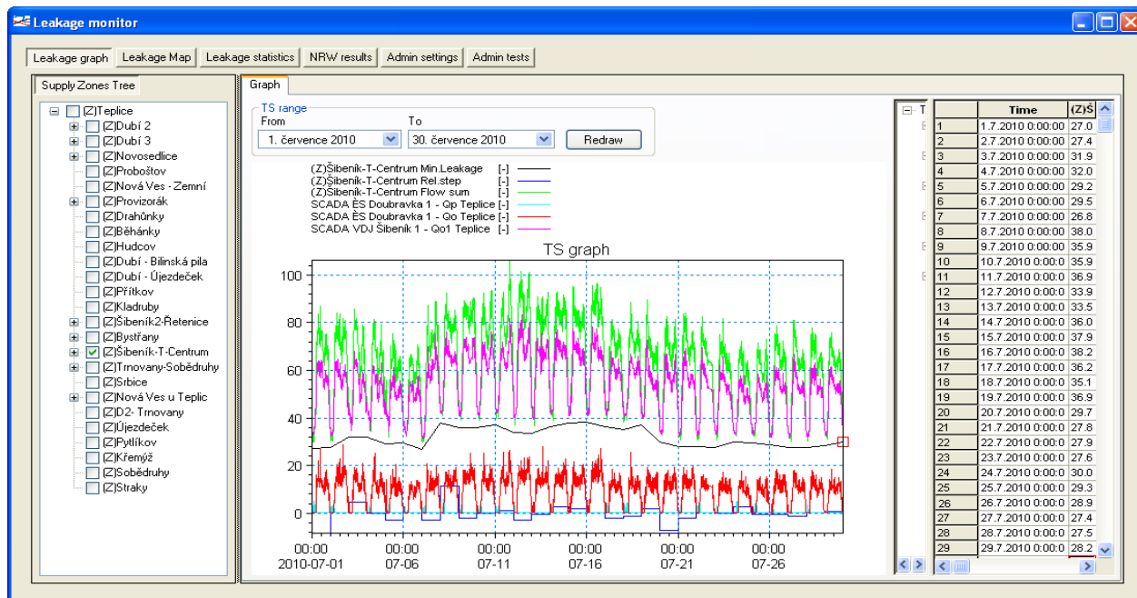
Figure 2 Automate evaluation of leakage (black line) from night inflow in a supply zone
