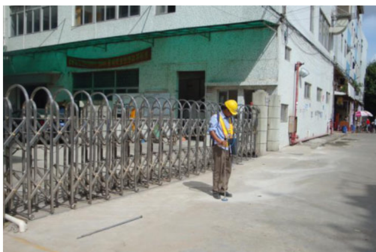
Figure 6 - Helium detection outside factory
